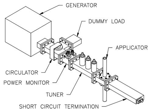
Figure 1. Typical laboratory system for fluid heating.
