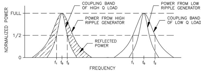
Figure 2. Generator output frequency spectrum compared to load coupling band.
