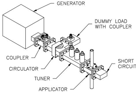
Figure 7. Basic heating system with coupler before isolator.
