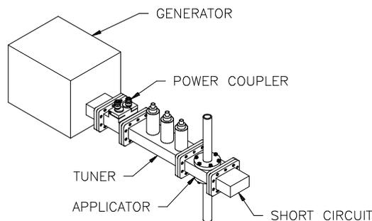
Figure 6. Basic heating system without isolator.
